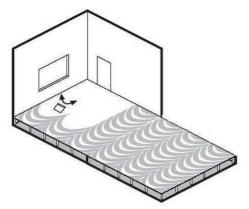
3. Lay the tiles starting along the centrelines and following the arrows printed on the back of the tiles taking special care to the alignment of joints. Cut the perimeter tiles to fit.
