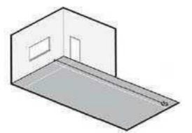
2. Loose lay the rolls (without adhesive) following the marked lines. Rolls must be laid with 3cm overlap along the adjoining edges. Check the uniformity of colour and the absence of defects.
