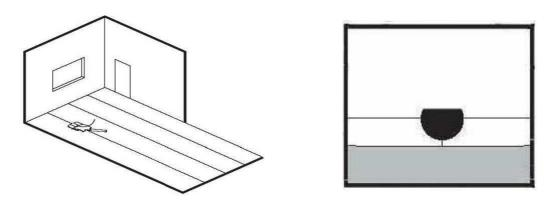
4. When the rod has cooled to room temperature the remaining excess should be trimmed using the spatula knife without the guide keeping a shallow angle between blade and floor to avoid "digging in" .Attention: the colour of the rod cannot be exactly the same of the floor.
