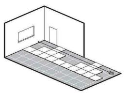
2. Loose lay the tiles (without adhesive)starting along the centrelines and following the arrows printed on the back of the tile staking special care to the alignment of joints and/or pattern.
