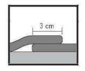
3. The loose laying is very important to check the colour uniformity and the absence of defects of the flooring. All claims will be accepted only if the flooring is not yet permanently bonded.
