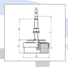
KFL machine feet have been designed with ease of installation in mind, this means that there is no need to fix the mount directly to the floor using bolts. The bonded rubber element means the KFL can withstand higher shear and compression loads, all without affecting performance.
